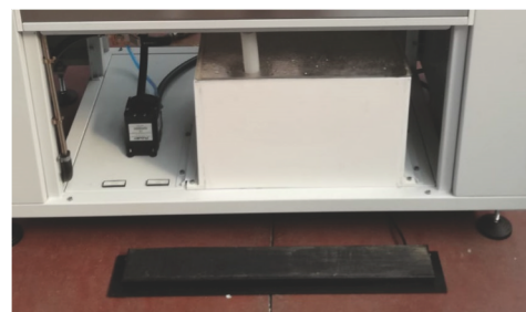
Safety pedal for manual operations
