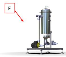
An external recycle device for washout water is available at request. It allows, thanks to a replaceable filter bag, to ensure most of the polymer washed from plates remains in the filter as well as black mask if digital plates are processed.
