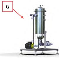
An external recycle device for washout water is available at request. It allows, thanks to a filter bag, to ensure that most of the polymer washed from plates remains in the filter as well as black mask if digital plates are processed.
